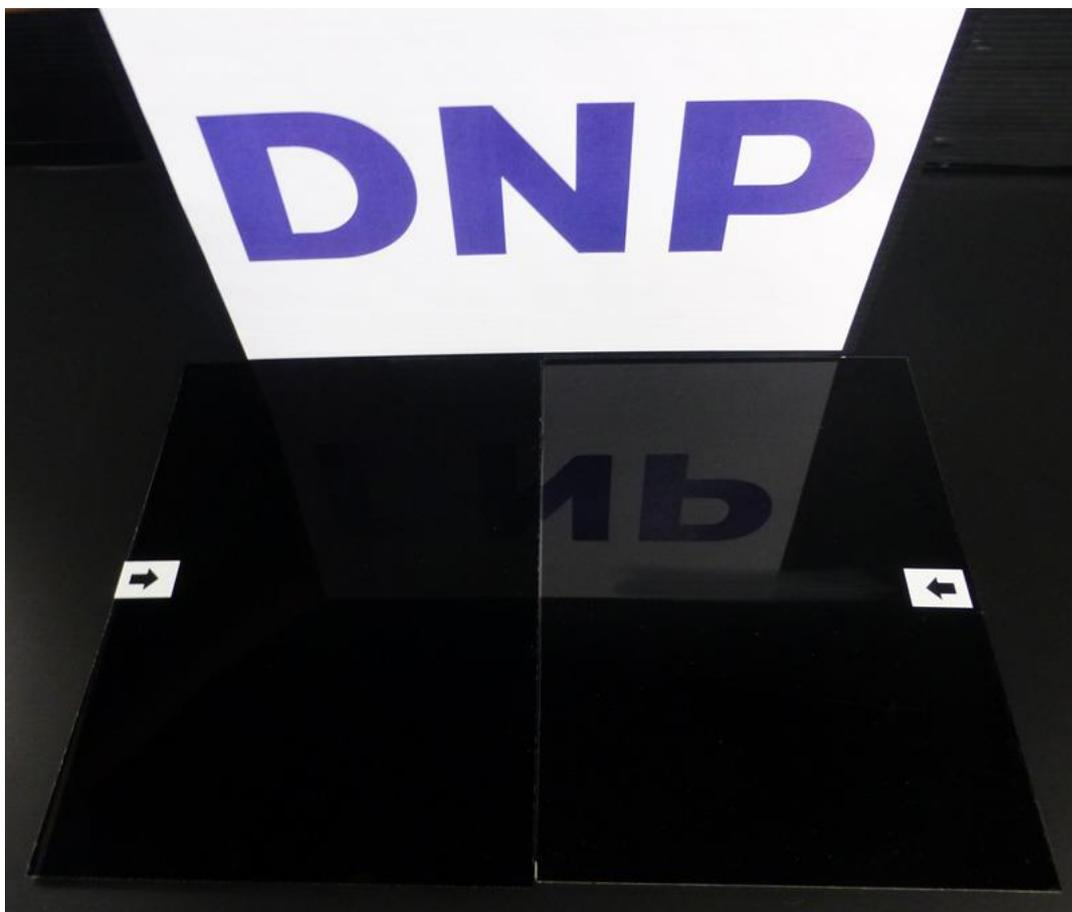
Compared to the conventional product (right) of DNP, it can be seen that the new product (left) does not show reflected characters. Also, with the new product (left), it can be seen that no damage occurs in the arrow portion.
